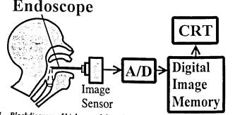
Figure 1 Blockdiagram of high-speed digital image recording system.
