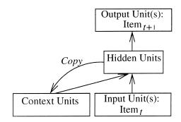
Figure 1. Architecture of the simple recurrent network (SRN).
